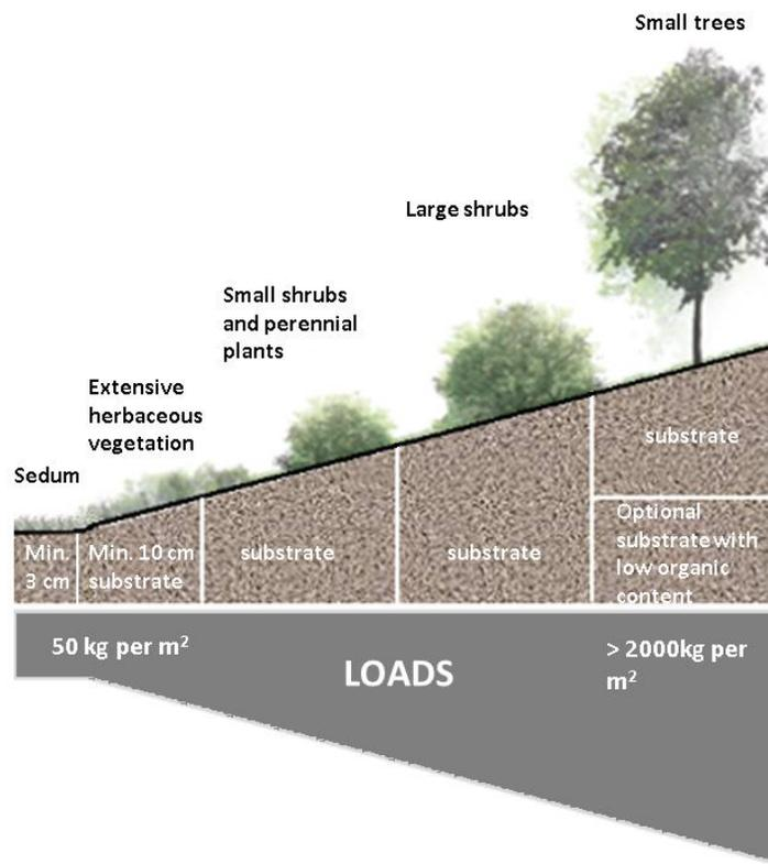
**Fig. 3.** Function of vegetation types relating to installation depths, giving different loads on the supporting concrete deck.
