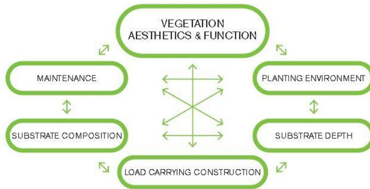
**Fig. 2.** Factors and relationships affecting the vegetative superstructures' appearance, durability and function but also the concrete structure, e.g. load carrying capacity. Changes in one factor may have great impact on other factors and on the system as a whole.
